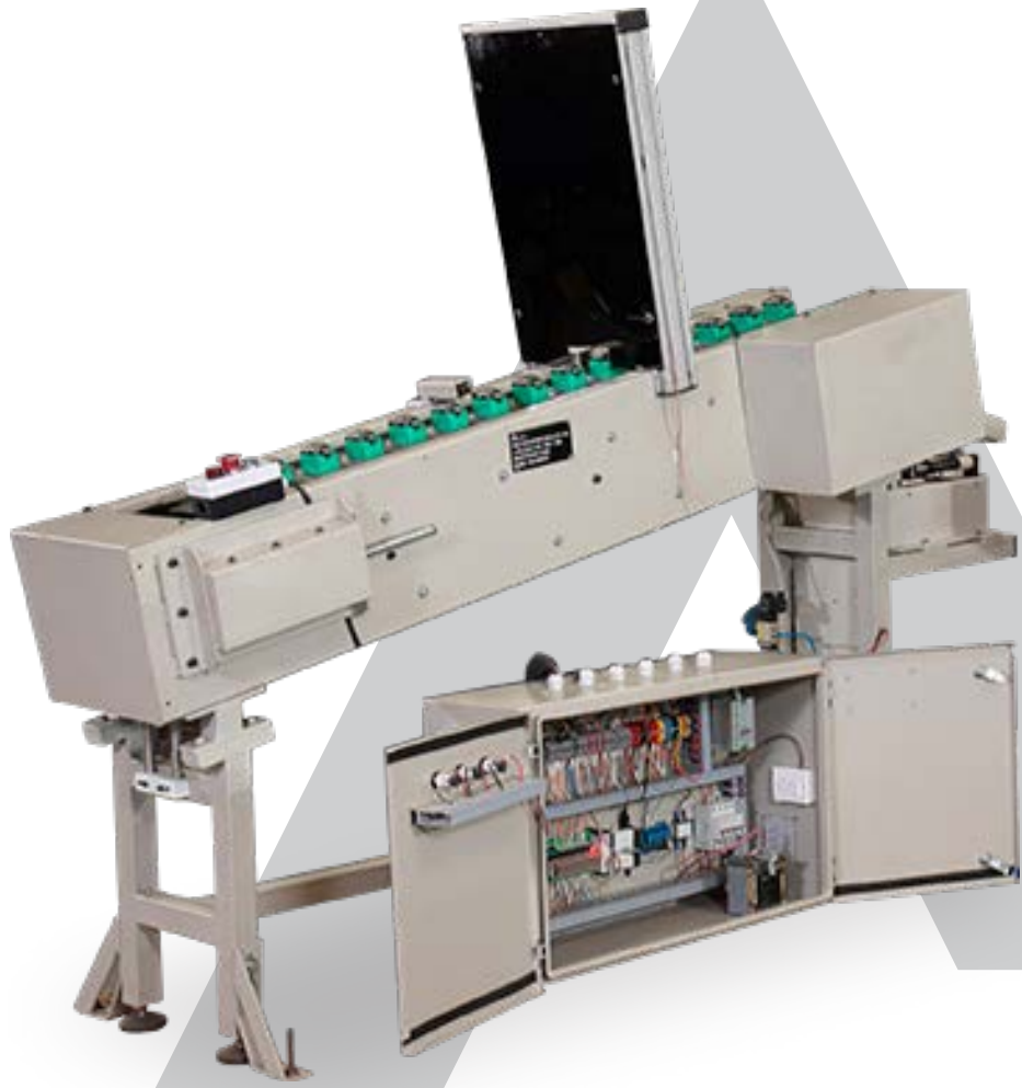
Conveyorised Camshaft Automatic Inspection Station
